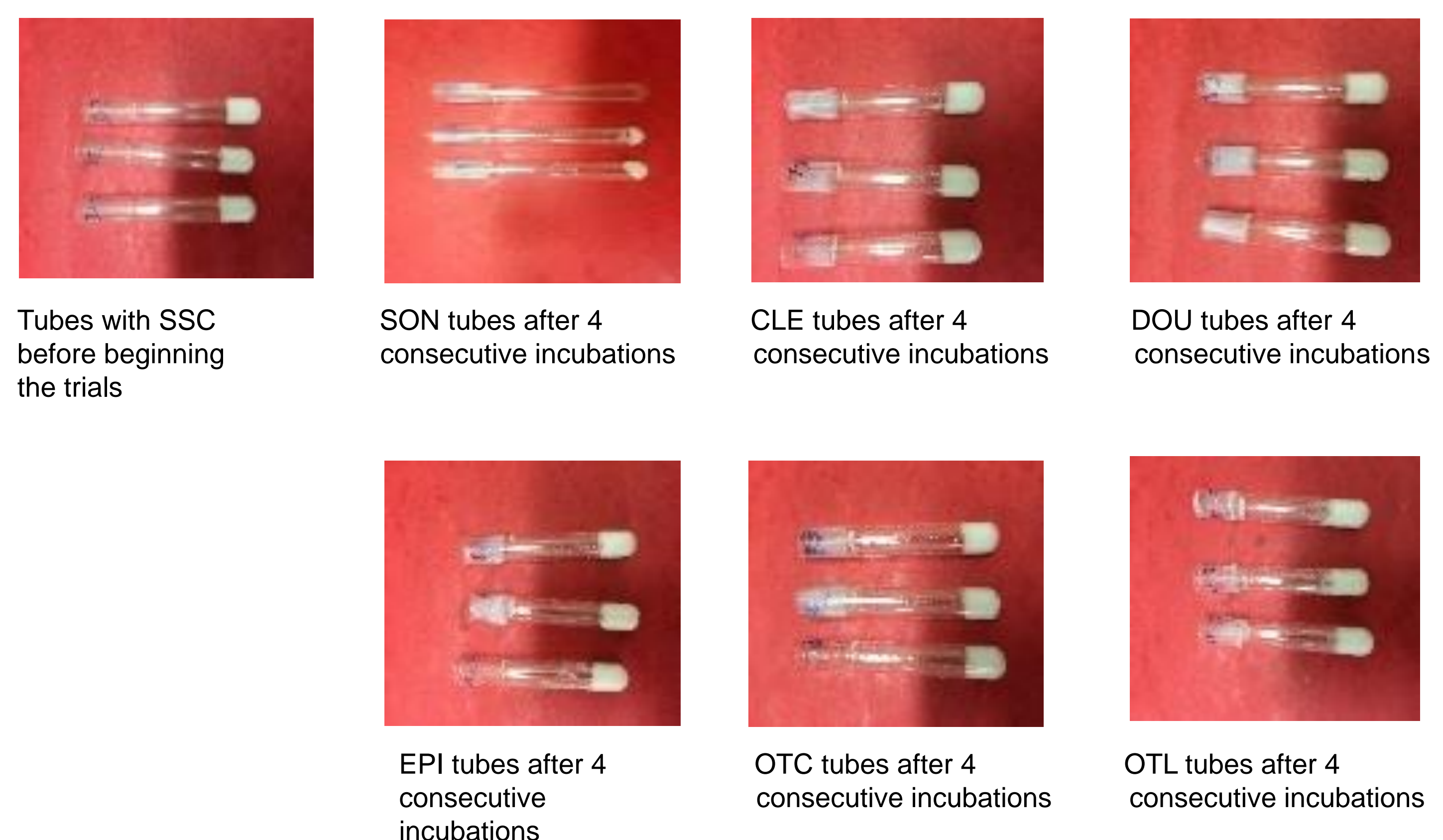
Figure 2 - Appearance of a selection of the tubes after four consecutive incubations showing different degrees of standardized synthetic cerumen (SSC) disintegration. As describe in Table 1, only SON induced an increasing degree of SSC disintegration and removal whereas the 5 other products didn't show any effect on the SSC plug.
